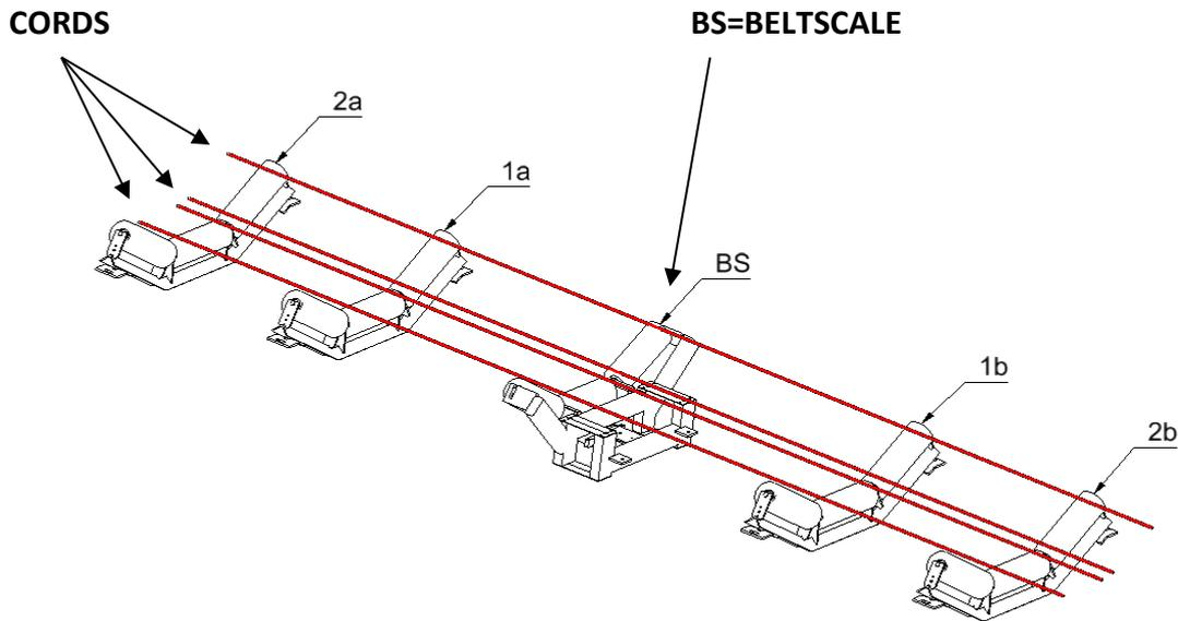
The distance from roll 1a/ 1b and the center of the belt scale roller must be carefully measured from the center of the belt weigher roll and preferably not less than 1000mm.
