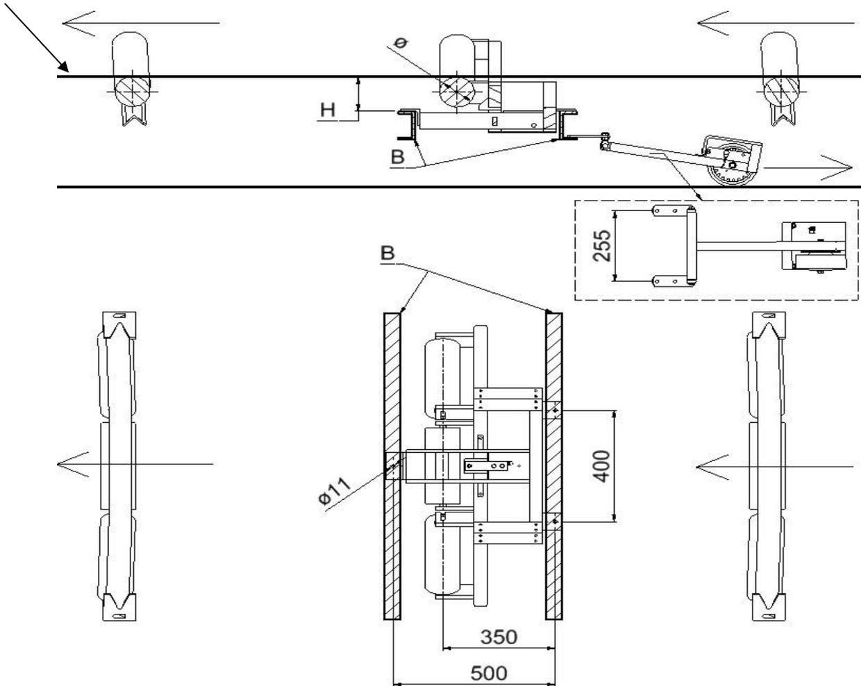
H = Distance from measuring line top of middle roller to top of mountingframe.
