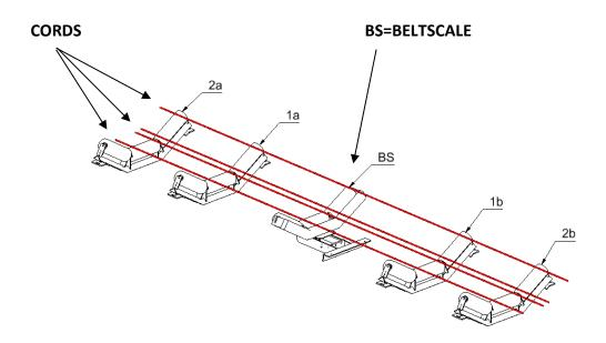
The distance from roll 1a/ 1b and the center of the belt scale roller must be carefully measured from the center of the belt weigher roll and preferably not less than 1000mm.
