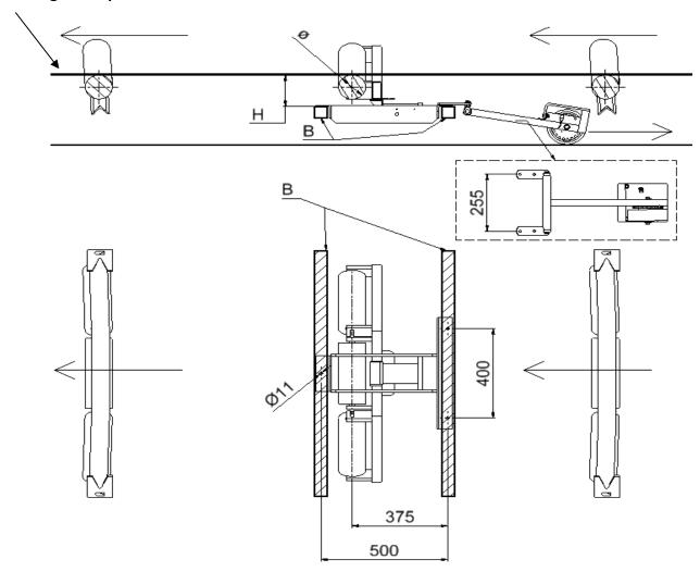
H = Distance from measuring line top of middle roller to top of mountingframe.
